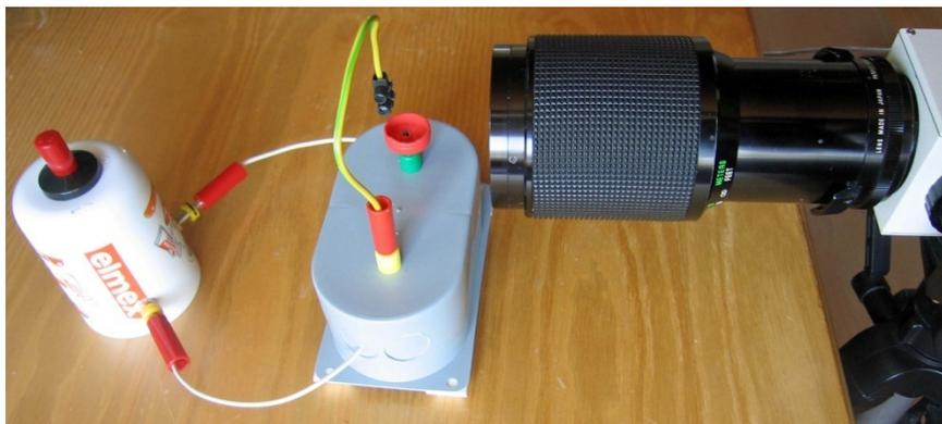
Logically, during the spark discharge the part of the generated plasma is recorded, which is located just on the slit of the spectrograph. Therefore, the impact point of the spark on the sample must be centered on the slit as precisely as possible. Preferred impact points are sharp tips, corners or edges.
