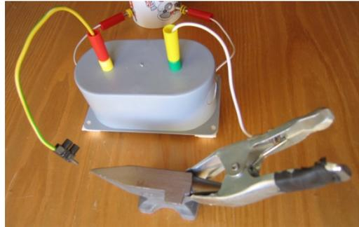
Who plans more extensive tests will probably better use a spark inductor. This may be constructed for example using a simple car ignition coil and some additional electronics, which nowadays replaces the former terribly rattling mechanical interruptor. Under these keywords numerous construction guidances are to find on the Internet.
